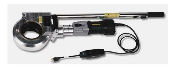
The machine operates on either 110 V or 220 V power. It is a single-direction operator; to change directions, take the operator off the valve key and turn it over. It is not designed for the back-and-forth valve exercising performed by the WAVE handheld or Power Drive 11 operators.
