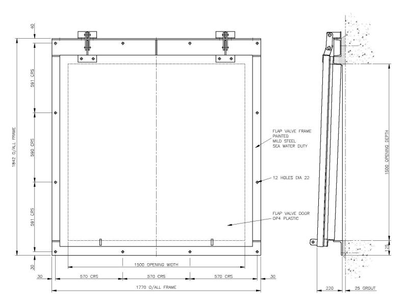
Typical Drawing only of a Rectangular Fabricated Flap Valve. Painted Mild Steel Frame and HDPE Door. Size 1500 x 1500
