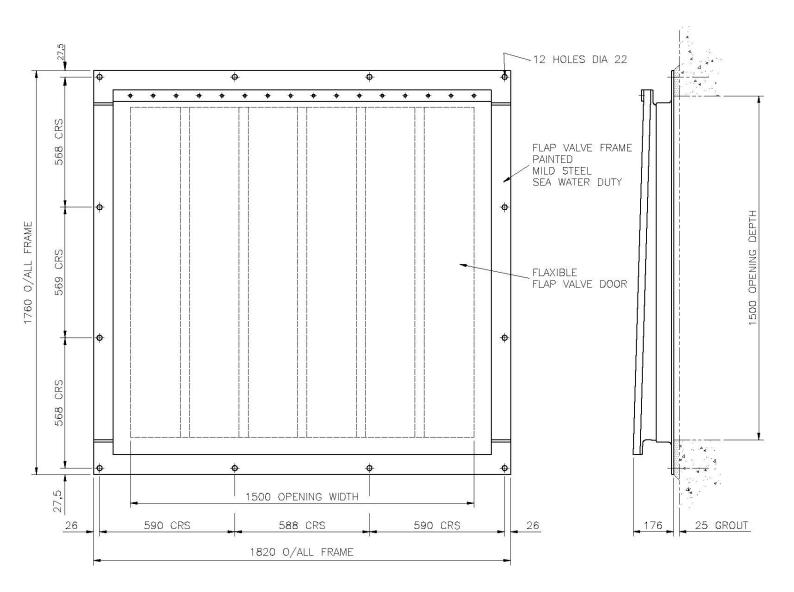
Typical Drawing only of a Rectangular Fabricated Flap Valve. Painted Mild Steel Frame and Rubber Door. Size 1500 x 1500
